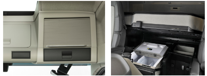
DIN slots and storage units above the windscreen and under-bunk storage units.
